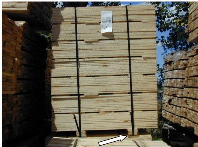
**Figure 2 - Dunnage used in sawn wood shipments**
