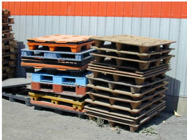
**Figure 10** - Plastic and fibre-form pallets
