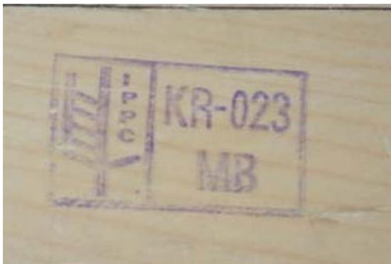
**Figure 3<sup>6</sup>** – Mark matches example 1 of Annex 2 of ISPM 15:2009.
