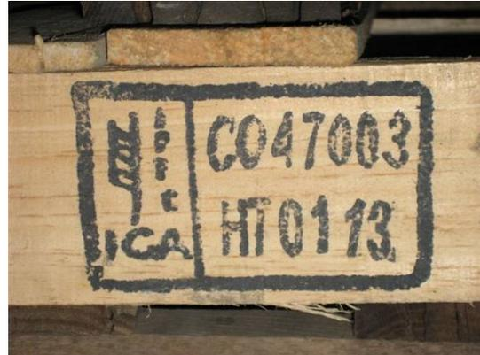
**Figure 2<sup>6</sup>** – Information beyond what is prescribed in Annex 2 of ISPM 15:2009 contained within the borders of the mark.
